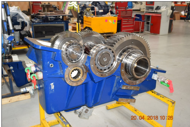
Wind Turbine Gearbox, Ireland
