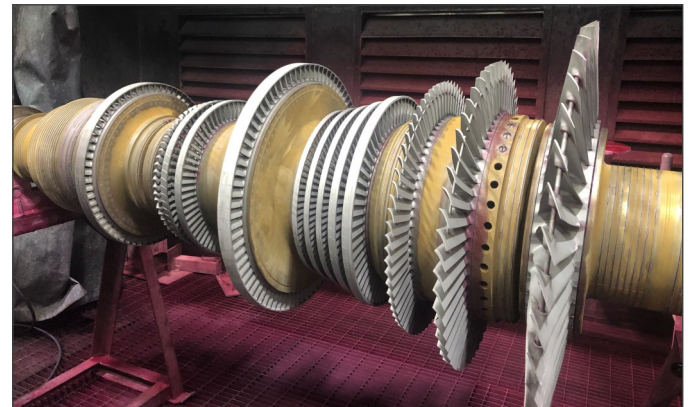
Steam Turbine Rotor
